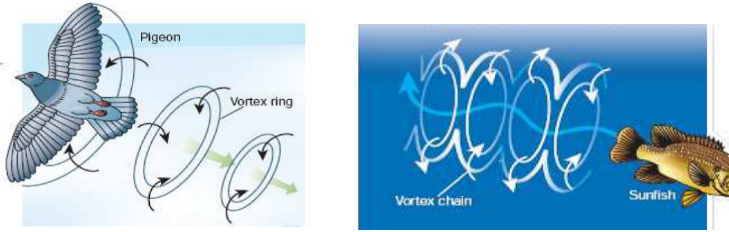
Figure 2. Locomotion in fluids and vortical structure generated at each stroke by bird and fish (Pinheiro, 2010).
